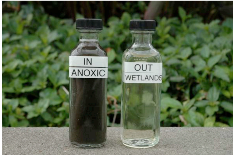
Influent and effluent from the Living Machine
